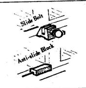
Slide blocks or slide bolts should be used to prevent doors and windows from being lifted out of the track.
