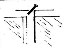
These windows can be made secure by drilling a downward sloping hole through the first sash, and one into (but not through) the second sash. Slide a nail or dowel into the hole.
