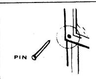
A nail or metal pin without a head can be slid into a downward sloping hole that has been drilled into overlapping frames. A headless nail or pin can not be pulled out if the glass is broken out.
